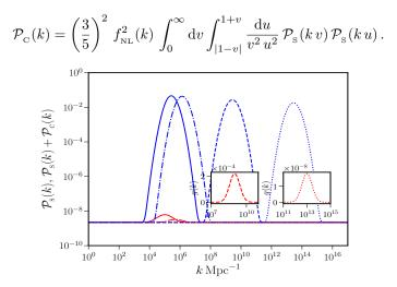
The corrected power spectra (in blue) against the original spectra (in red).
